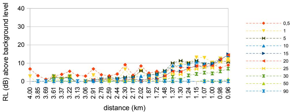
**Figure 3:** RL (in dB) measurements above background level for selected frequency bands (0.5-90 kHz) during approaches from a 4 km distance to CPA for the (a) fast ferry, (b) regular ferry and (c) high-speed ferry with the hydrophone suspended to 15 m.
